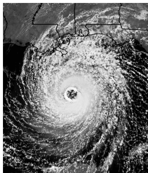
Above: Simulated image of ABI Band 3 (0.86 \mu\text{m} ) for Hurricane Katrina. This image was simulated via a combination of high spatial resolution numerical model runs and advanced “forward” radiative transfer models. Credit: CIMSS
